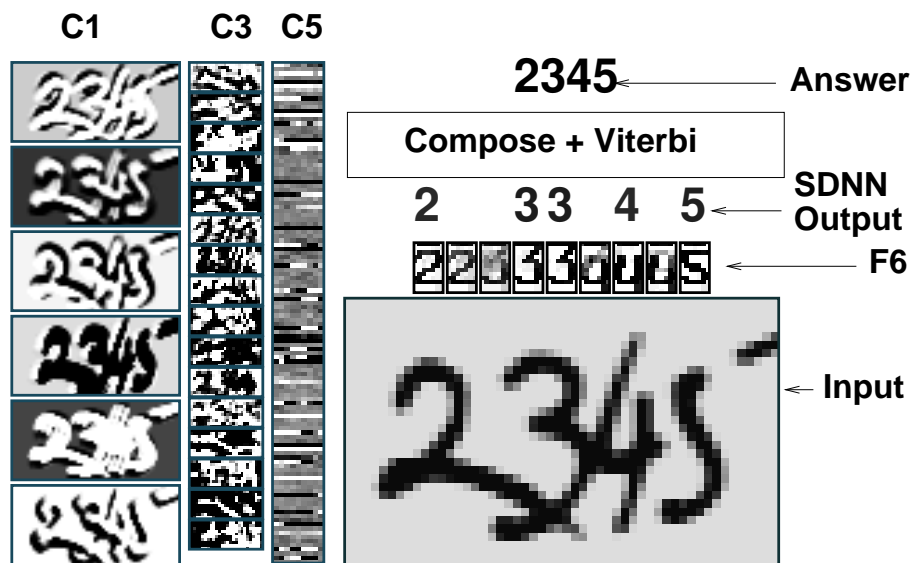
Figure 25: An example of multiple character recognition with SDNN. With SDNN, no explicit segmentation is performed.
