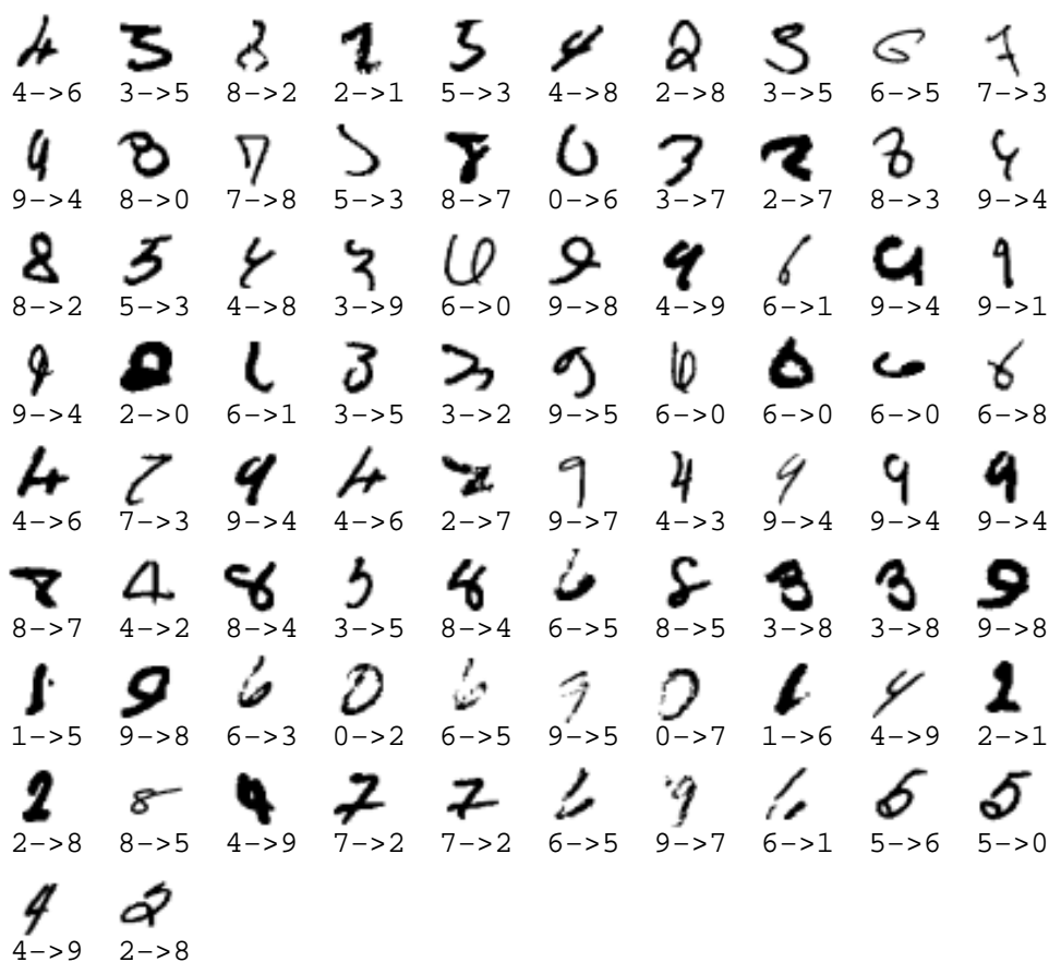
Figure 8: The 82 test patterns misclassified by LeNet-5. Below each image is displayed the correct answers (left) and the network answer (right). These errors are mostly caused either by genuinely ambiguous patterns, or by digits written in a style that are under-represented in the training set.
